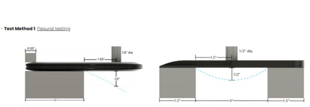
(1.1) Cantilever beam bending test
