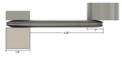
(2.1) Cantilever beam bending fatigue test
