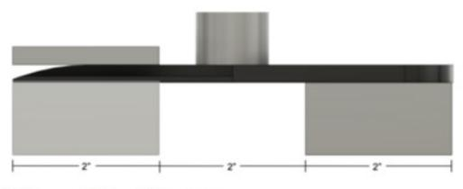
(22) Three-point flexural fatigue test
