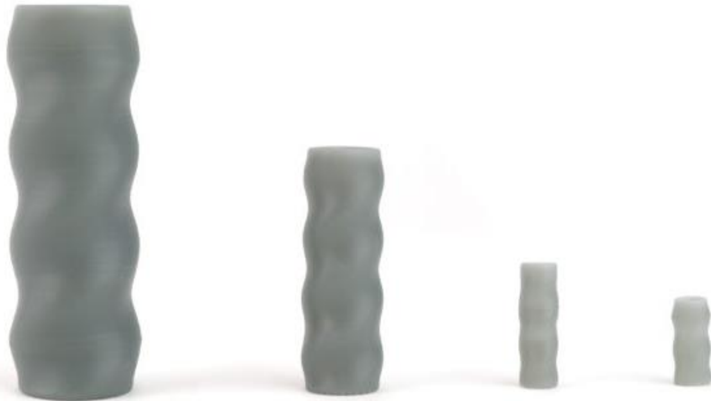
Figure 1: Different sizes of 3D printed airway stents, produced using Carbon printers and SIL 30
