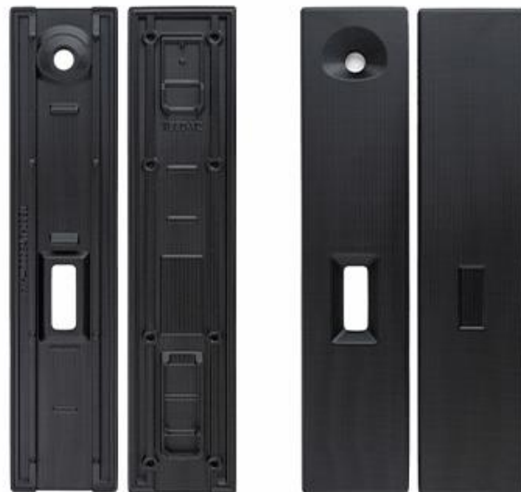
Figure 1: Tuberculosis diagnostic cassette, 3D manufactured using Carbon technology
