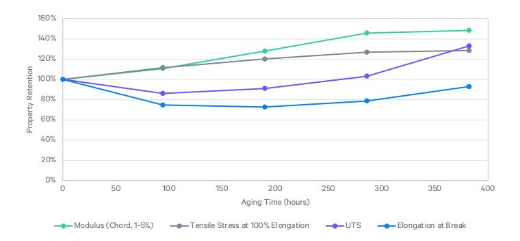
ASTM D4459: Q-Sun XE-1, 0.8 W/m<sup>2</sup>/nm at 420 nm, 55 °C ASTM D412: Die C, 500 mm/min, average values represented
