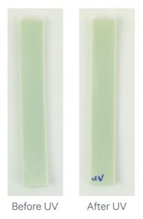
ISO 4892-1/4892-2: Xenon-arc lamp, UV-Quartz filter, 1.2 W/m $^2$ /nm, at 420 nm, 70 °C, 6 hours
