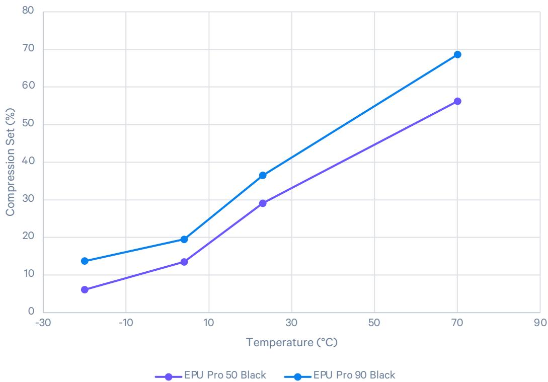
Parts were processed using an L series printer and centrifugal spinner (EPU Pro 90 Black) or PGDA wash followed by IPA wash (EPU Pro 50 Black). The cleaned parts were cured and baked following the EPU Pro 50 and 90 Black standard workflow curing and baking schedule.
