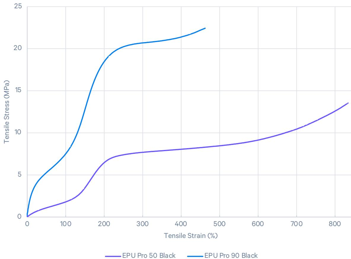
Parts were processed using an L series printer and centrifugal spinner (EPU Pro 90 Black) or PGDA wash followed by IPA wash (EPU Pro 50 Black). The cleaned parts were cured and baked following the EPU Pro 50 and 90 Black standard workflow curing and baking schedule.
