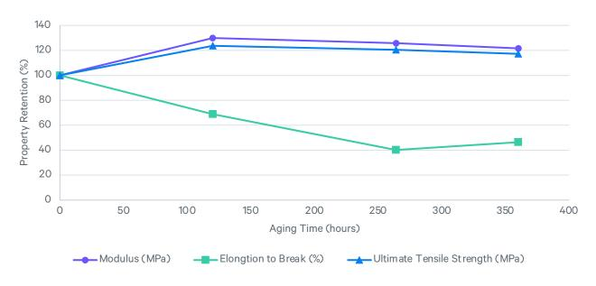
ASTM D4459: Q-Sun XE-1, 0.8 W/m<sup>2</sup> at 420 nm, 55 °C ASTM D638: Type V, 500 mm/min, average values represented
