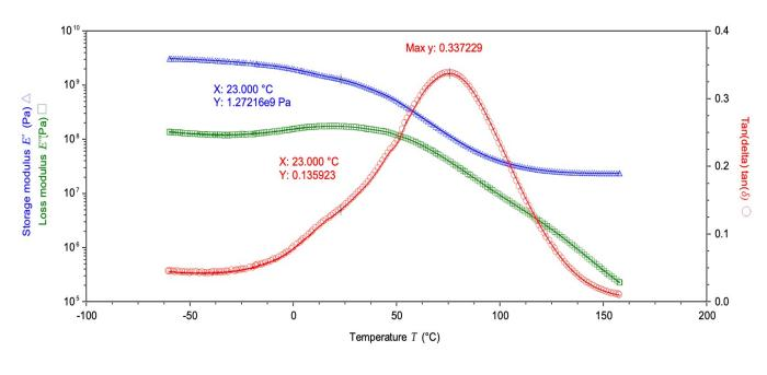
Standard: ASTM D4065 Instrument: TA DMA Q800 DMA Mode: Tension Sample Dimensions: L=20 mm, W=10 mm, t=1 mm (rectangular block) Strain Amplitude: 0.1% (linear regime of viscoelasticity) Oscillation frequency: 1 Hz Temperature Range: -60 °C to 150 °C Ramp Rate: 1.5 °C/min
