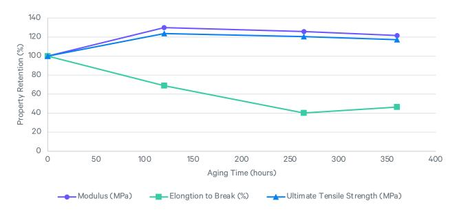
ASTM D4459: Q-Sun XE-1, 0.8 W/m² at 420 nm, 55 °C ASTM D638: Type V, 500 mm/min, average values represented
