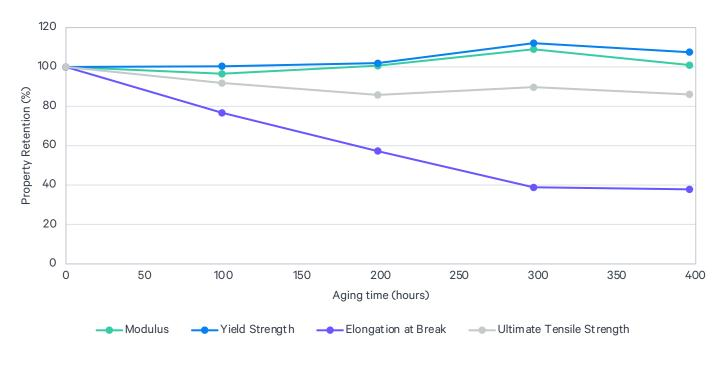
ASTM D4459: Q-Sun XE-1, 0.8 W/m²/nm at 420 nm, 55  $^{\circ}\mathrm{C}$  ASTM D638: Type V, 10 mm/min, average values represented
