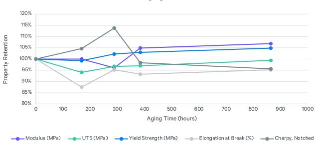
ASTM D638: Type I, 50 mm/min ISO 179-1/1eA: Notched Charpy (Machined Notch)
