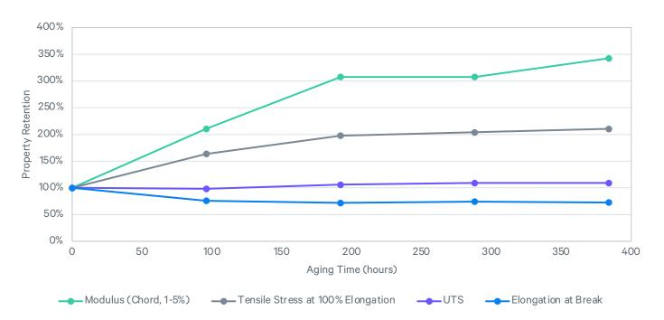
ASTM D4459: Q-Sun XE-1, 0.8 W/m² at 420 nm, 55  $^{\circ}\text{C}$  ASTM D412: Die C, 500 mm/min, average values represented
