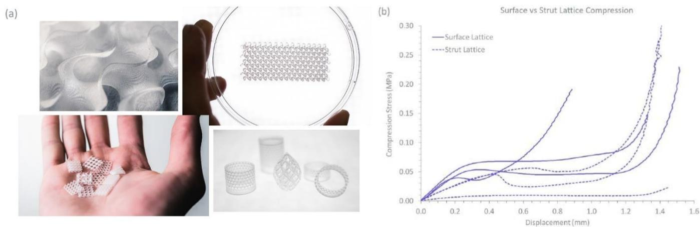
**Figure 4. (a) Surface and strut-based lattice geometries have been printed on the Carbon M2 series with high resolution. Parts pictured were designed with wall thicknesses  $\sim 180\text{-}250\ \mu\text{m}$  wide. (b) Using DLS technology, Carbon can print a variety of strut-based and surface lattices to obtain various compression profiles using the same BE resin.**
