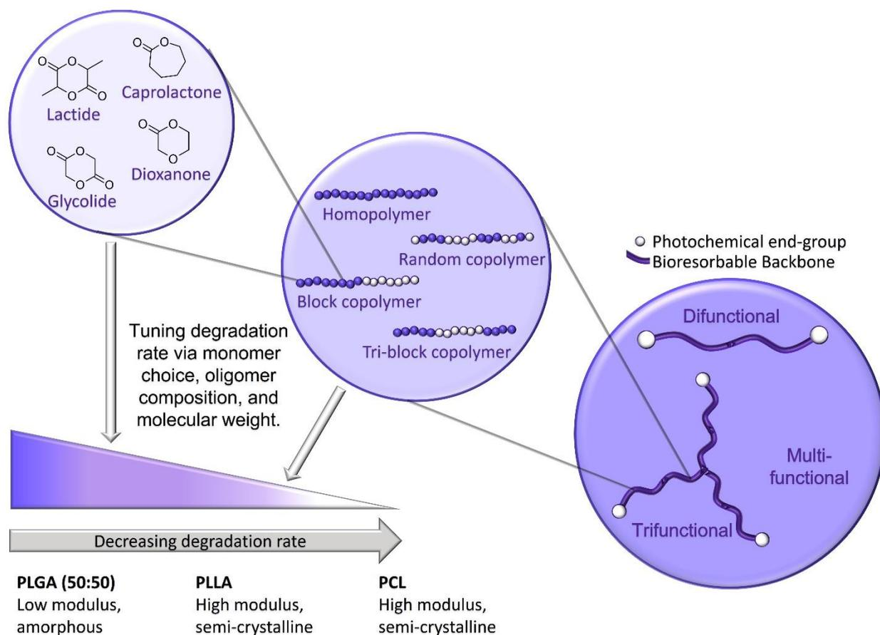
Figure 1. ATPEs are the main component of Carbon's bioabsorbable resin platform. The ATPEs are linear or branched, methacrylate-terminated polyester oligomers that vary in molecular weight, oligomer composition, and monomer backbone which allows for tunability of degradation rate without sacrificing elastomeric properties.
